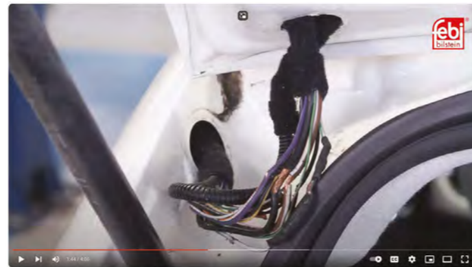
[EN] Fiat 500 tailgate wiring harness repair
