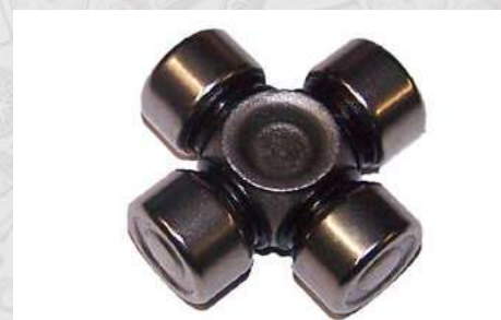
Universal Joint Part No: 749-0024 Application: Mercedes Vito 03 >, Sprinter 06 >
